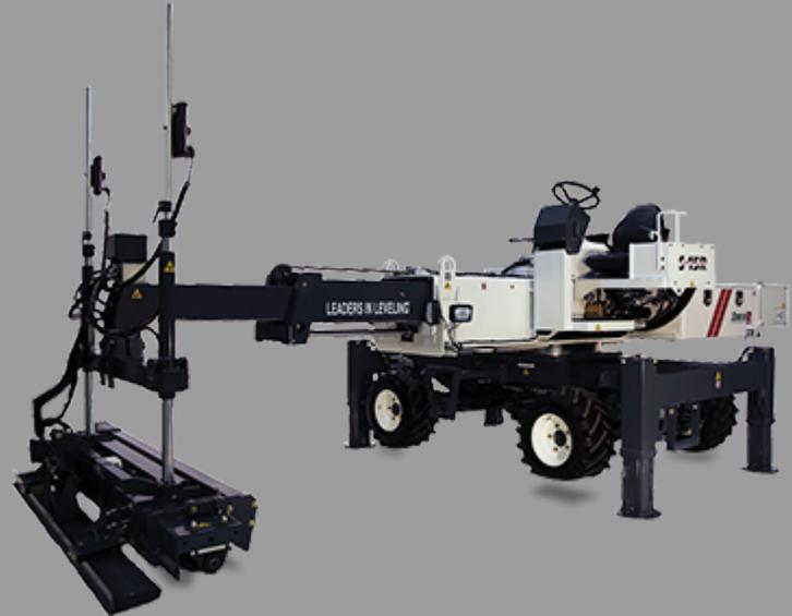
The S-15R features a fully integrated OASIS laser control system which allows the screed head to hold grade while it levels and consolidates the concrete in a single pass. The hardened, double flight auger cuts the concrete to grade and displaces excess concrete to the side while the offset head design minimizes overlap giving you more screeded concrete in one pass.
